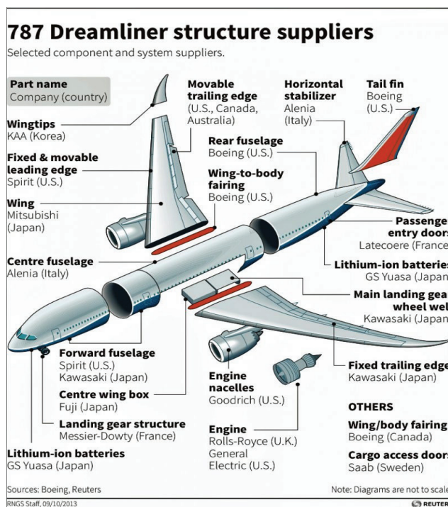
Source: REUTERS GRAPHICS; Diagram of the Boeing 787 with details parts and where they are manufactured.
